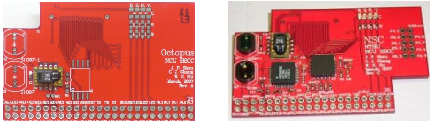
Sensor Board Size: 50mm × 31mm
